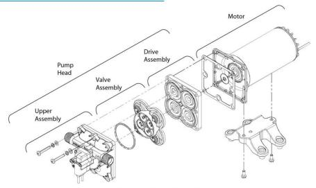
Pressure Switch and Check Valve not shown
